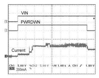
Figure 31. Power Up / Boot Up Current Waveform
